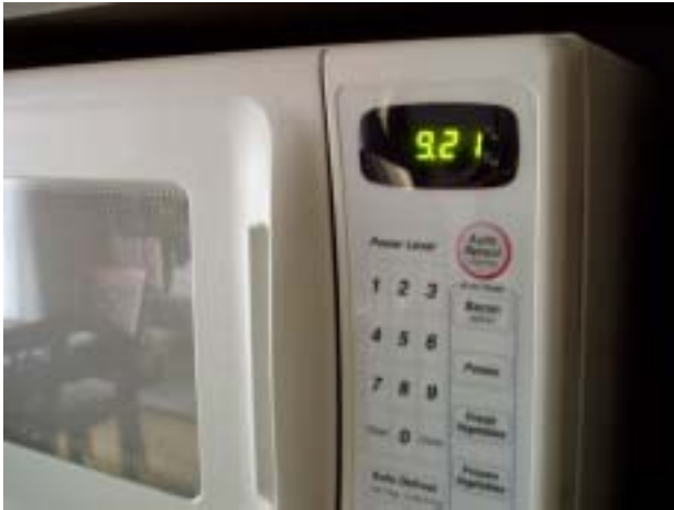
Figure 19. Phantom loads are unnoticed and often useless electrical loads that burn holes in your energy conservation plan. Examples are doorbells, “instant on” electronics and microwave ovens or anything that uses a “power adapter”, like the one shown above.
