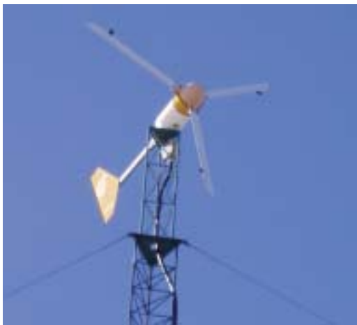
Figure 12. With advances in materials technology, you will find wind power used in every location on earth. The Bergey 1500 small wind turbine is specifically designed for home sized off-grid and grid-interconnected applications.
