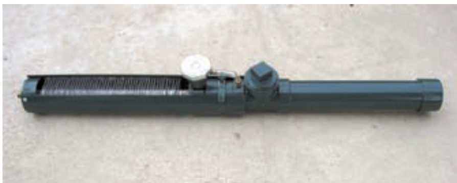
A TPFRS unit showing the radiator on the left, automobile radiator cap in the middle, and the overflow reservoir on the right.
